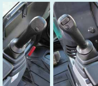
Proportional hand control lever for N&B piping (option)
